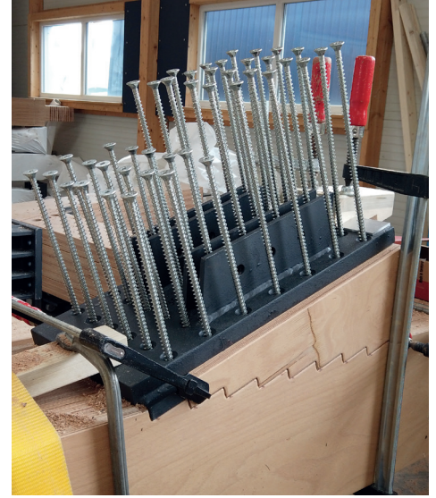
▲ Using BauBuche requires the use of special screws that have been approved for BauBuche. (Photo credit: SWG Schraubwerk Gaisbach GmbH – Production Division)
